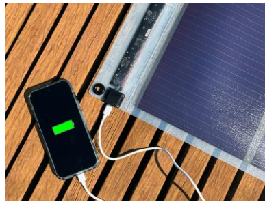
(2) Charging from Solar sheet to Mobile phone
